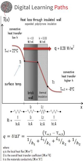
$$\dot{Q}_{wall} = -\frac{T_{\infty,1} - T_{\infty,3}}{R_{total}} = -\frac{T_{\infty,1} - T_{\infty,3}}{R_{\infty,1} + R_1 + R_2 + R_1 + R_{1,\infty}}$$
